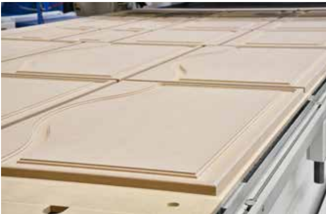
Optimal work piece holding with the high capacity vacuum up to 1000 m 3 /h.
